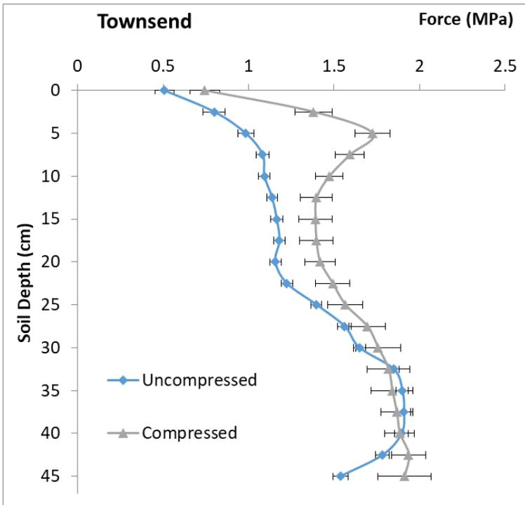
Figure 7-1 Penetration resistance profile measured in September 2019 (soil moisture at 23%)
