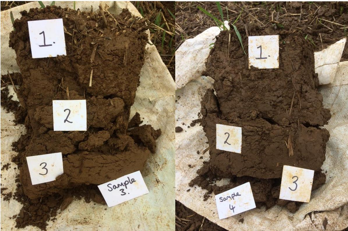
Figure 7-3 Example VESS profiles from a compressed plot (left) and a non-compressed plot (right). Numbers show location of VESS layers.
