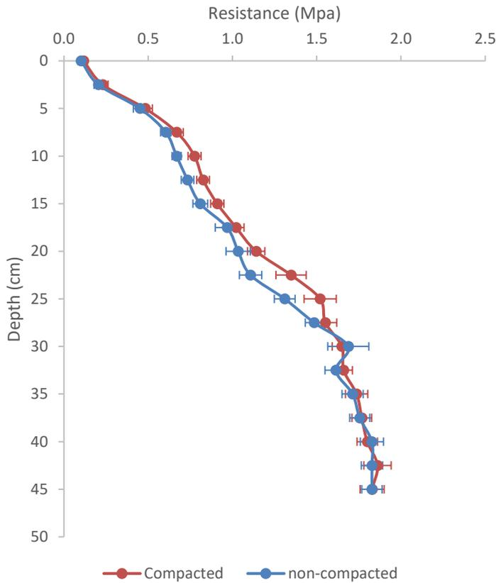
Figure 7-4 Penetration resistance profile, November 2020 (50% moisture – compacted plots; 35% moisture – non-compacted)
